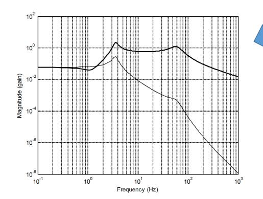
[A,B,C,D] = linmod('drive4'); sys = ss(A,B,C,D); f = [0.1:0.1:1000]'; [mag,phase] = bode(sys,f\*2\*pi); mag = squeeze(mag)'; loglog(f,mag); grid on;
